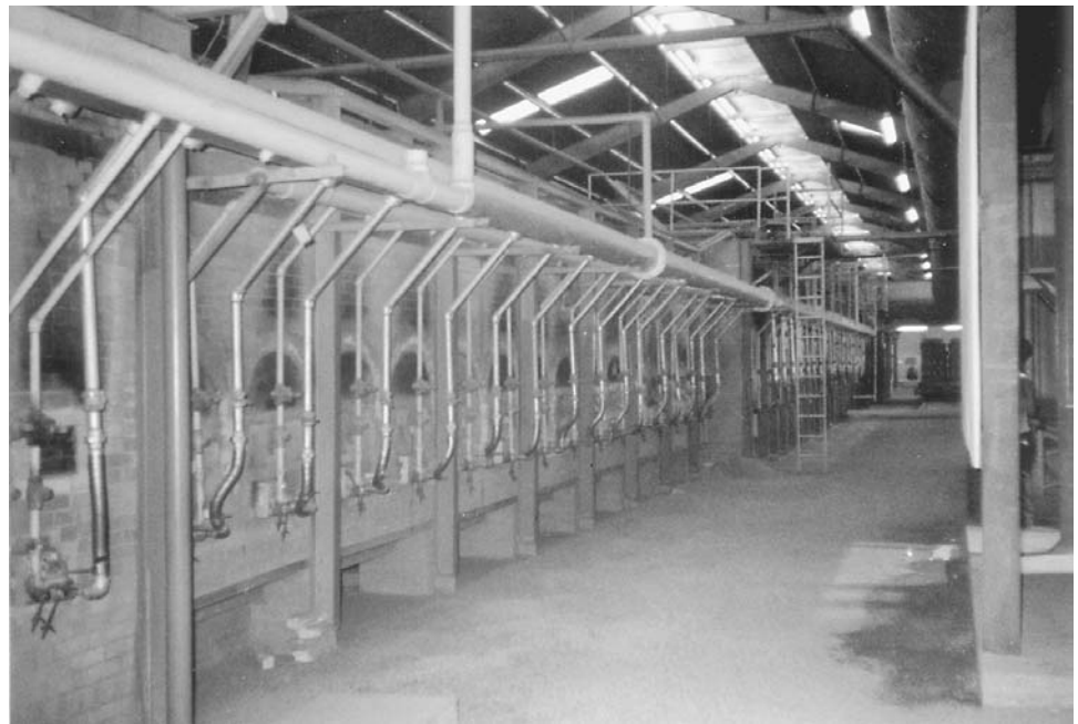
Figure 2-5 Tunnel kilns provide even heat distribution.
